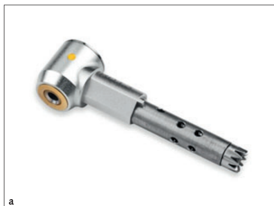
Fig 4 RDT hand-piece heads. The RDT handpiece head is used to turn the rotation of the micromotor into in-and-out vibrations. It also contains a special clutch mechanism. Such heads are available for connection to a KaVo type handpiece: RDT3 (a) or RDTNX (b), which can be used with any NSK-type connector, such as those used by the X-smart machine (Dentsply Maillefer).
