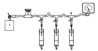
FIG 2. The pressure manifold. The pressure manifold was constructed from intravenous infusion tubing and connectors. A compressed air source (1) was connected through a fine pressure regulator (2) to a manifold (3) and to a manometer. A pressure of 300 mm Hg was used to test the system for an air tight seal, under water, before use. In the second part of the study a constant pressure of 120 mm Hg was applied for 7 days.
