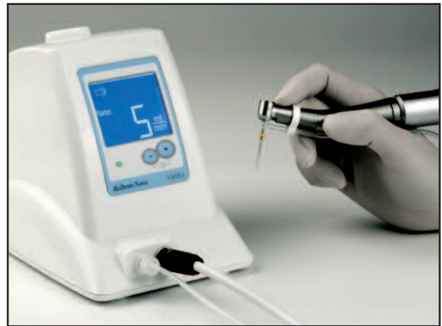
Fig. 7 VATEA peristaltic pump. The VATEA peristaltic pump, attached to the SAF via a silicone tube. The control panel is set at 5 mL/min.
