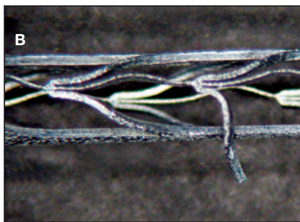
Fig. 15 Mechanical durability of the SAF. Durability of the SAF tested in a standard canal (block) using a setup (A) that simulates manual pecking motion by the movement of the asymmetric cam (*). The file was inspected at 1 min intervals for 29 min before any mechanical damage occurred. When such damage did occur, it was in the form of arch detachment (B). No file separation was encountered.
